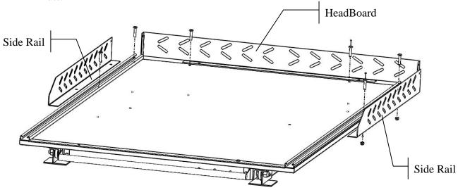
Connect side rail and head borad by M6s Bolt and Nuts.
